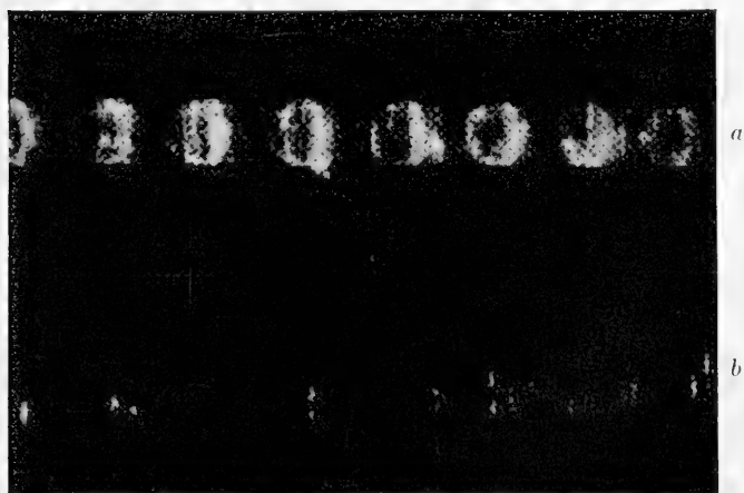
2. Radiograms of a metal surface after it has been rubbed with a piece of metal containing a radioactive component. The radioactivity of the surface shows there had been a transfer of material. This explains to a large extent the friction set up when one surface slides over another. The illustration relates to the friction of lead on steel: a , with no lubricant; b , with lubricant. Magnified about six times. (From J. N. Gregory, Nature (London) , vol. 157, p. 444, 1946.)
